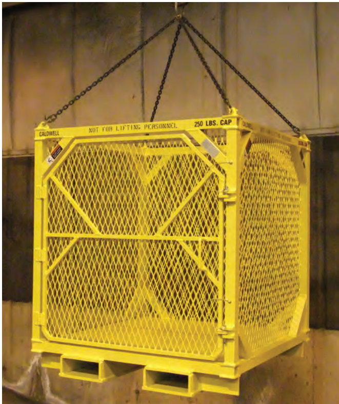
Heavy-duty steel with solid steel door and fork pockets.
